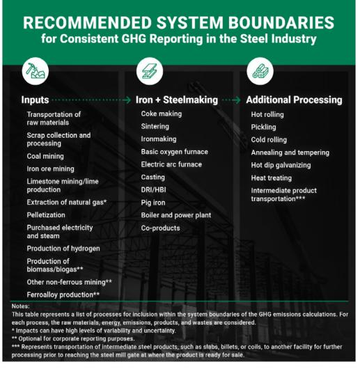
Figure 12: AISI's recommend system boundaries for GHG reporting in the steel industry (AISI, 2022d).
