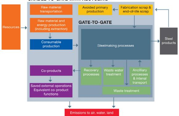
Figure 9: LCI Boundary for steel produced with scrap from the World Steel Association's LCI Methodology Report 2017 (World Steel Association, 2017).
