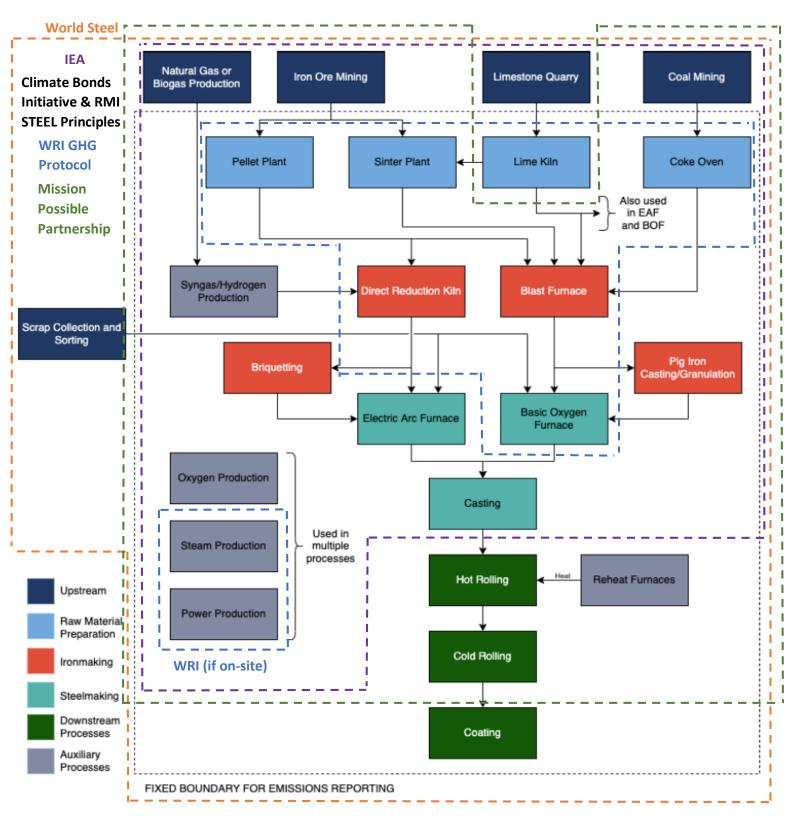
**Figure 2:** Comparison of system boundary of several steel decarbonization standards, protocols, and initiatives. (It should be noted that around 90% of CO2 emissions in primary steelmaking is related to ironmaking processes (blast furnace, sintering, coking), which are included in all system boundary shown in the figure.)
