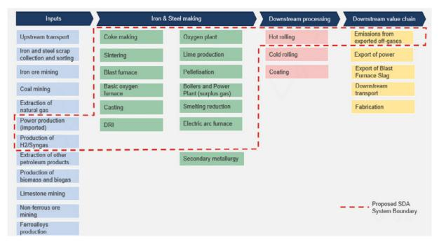
Figure 16: Iron and steel industry core SDA boundary proposed on the draft 1.5°C Steel Science-Based Target Setting Guidance.
