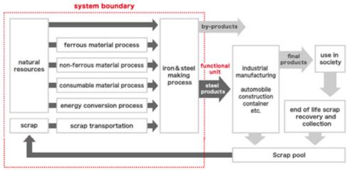
Figure 32 System boundary under JIS Q 20615 (The Japan Iron and Steel Federation, n.d.).
