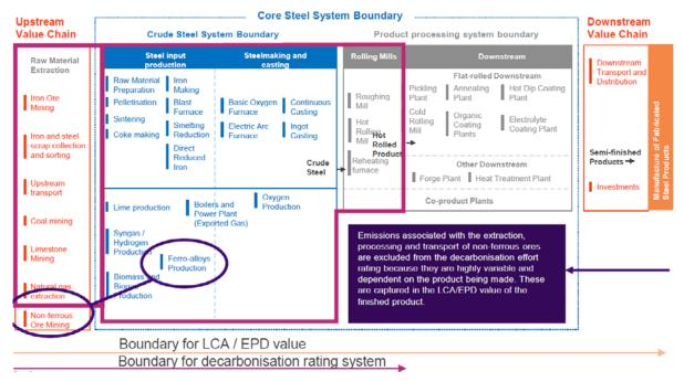
Figure 22: ArcelorMittal proposed system boundaries for their Low-Carbon Emissions Steel Standard (ArcelorMittal, 2022b).
