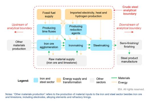
Figure 26: IEA's analytical boundary for defining near zero emission steel production (Levi et al., 2022).
