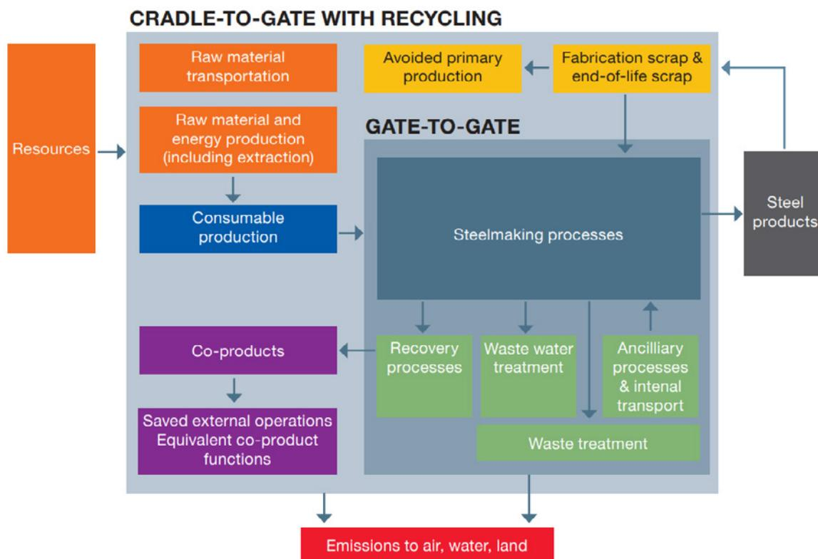
Figure 9: LCI Boundary for steel produced with scrap from the World Steel Association’s LCI Methodology Report 2017 (World Steel Association, 2017).
