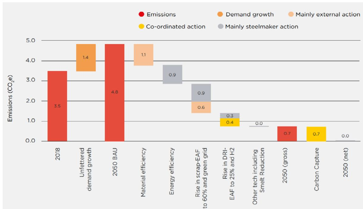
Figure 25: Major measures to reach net zero for the steel industry by 2050 and their projected contributions according to Climate Action 100+ (Gardiner & Lazuen, 2021).
