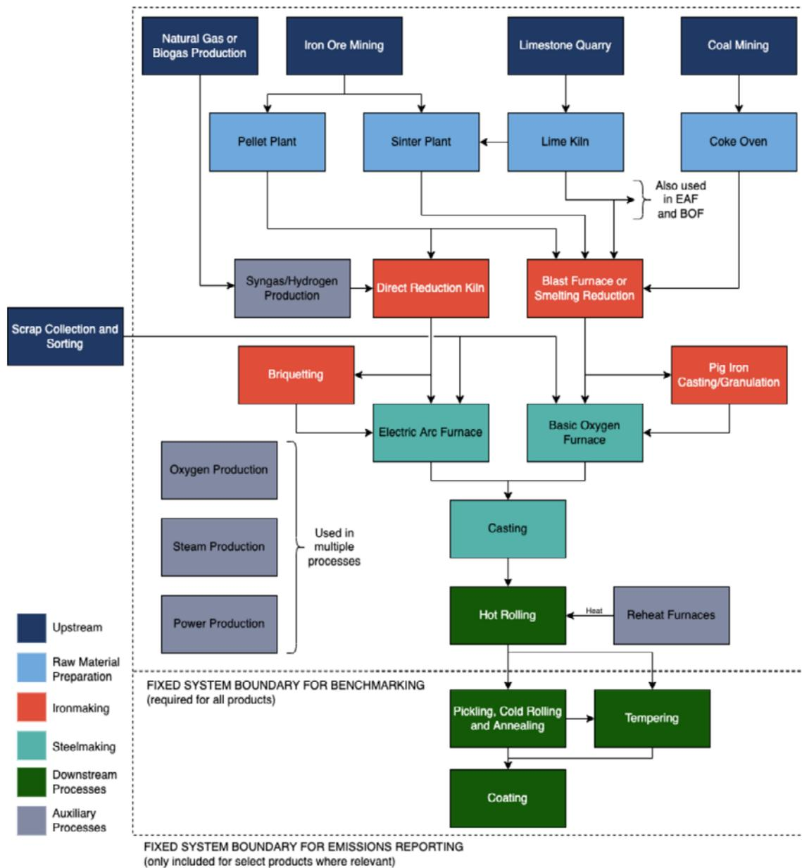
Figure 24: Emissions Reporting and Benchmarking boundaries for emissions in RMI's Steel Emissions Reporting Guidance (Wright, 2022)
