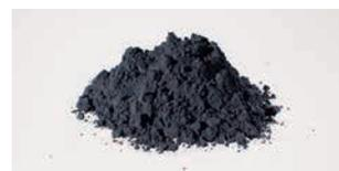
Lithium Nickel-Cobalt-Aluminum Oxide (NCA) used mainly in battery material (cathode material) for electric vehicles
