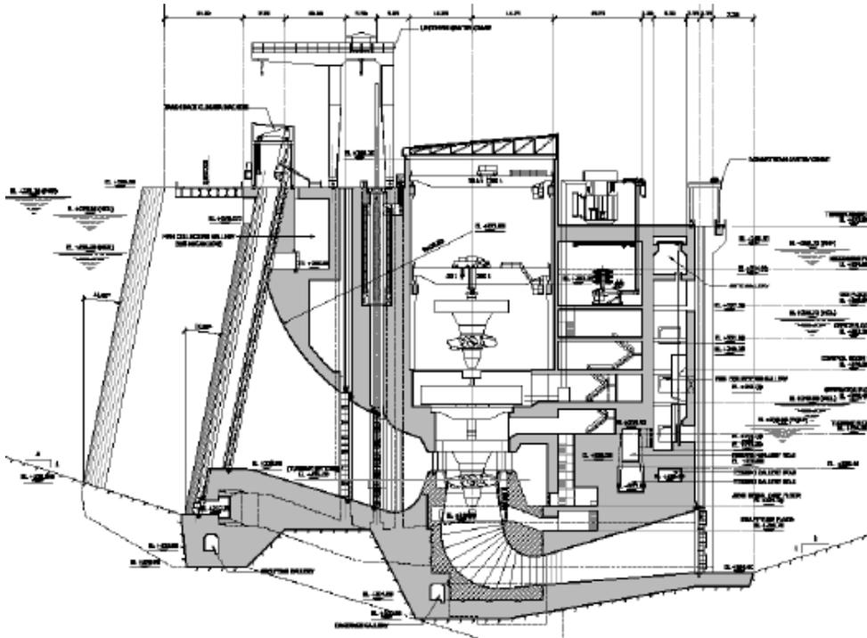
**Figure 3: Powerhouse cross section**
