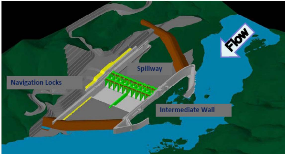
**Figure 5: First phase of construction proposed in the design documents**
