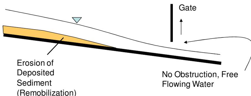
**Figure 12: Reservoir flushing operations to remobilise sediment already deposited require the presence of large capacity low-level outlets that can draw the river down to create free-flowing conditions at the dam. This flow condition re-mobilises sediment deposited and passes the re-suspended sediment downstream through the dam**
