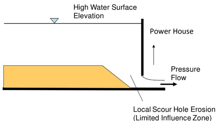
**Figure 10: Pressure flushing to remove localized sediment deposits**
