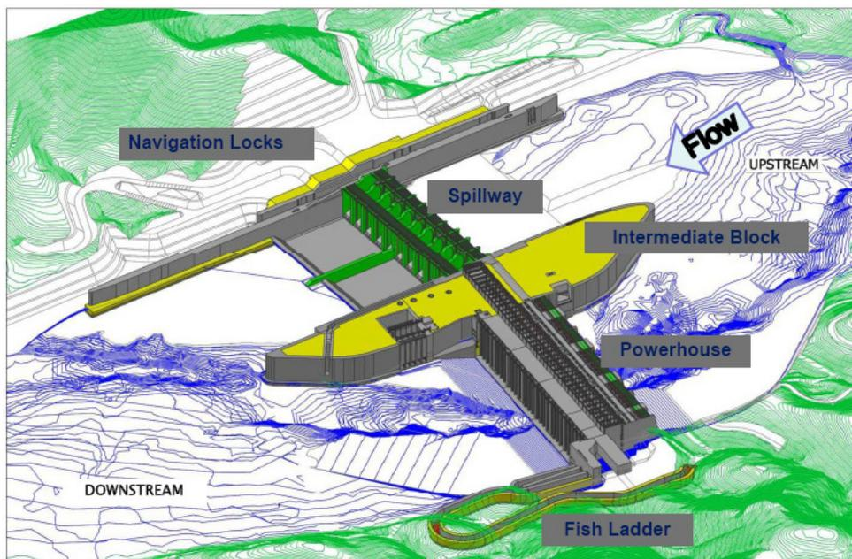
**Figure 2: Overall layout of Xayaburi dam project (Layout Report, 2010). The structure is 820 m long and 32.6 m high. The spillway facility comprises ten radial gates, 19 m wide and 21 m high. Gross reservoir volume is 1,300 m<sup>3</sup> or 1.3 km<sup>3</sup>**
