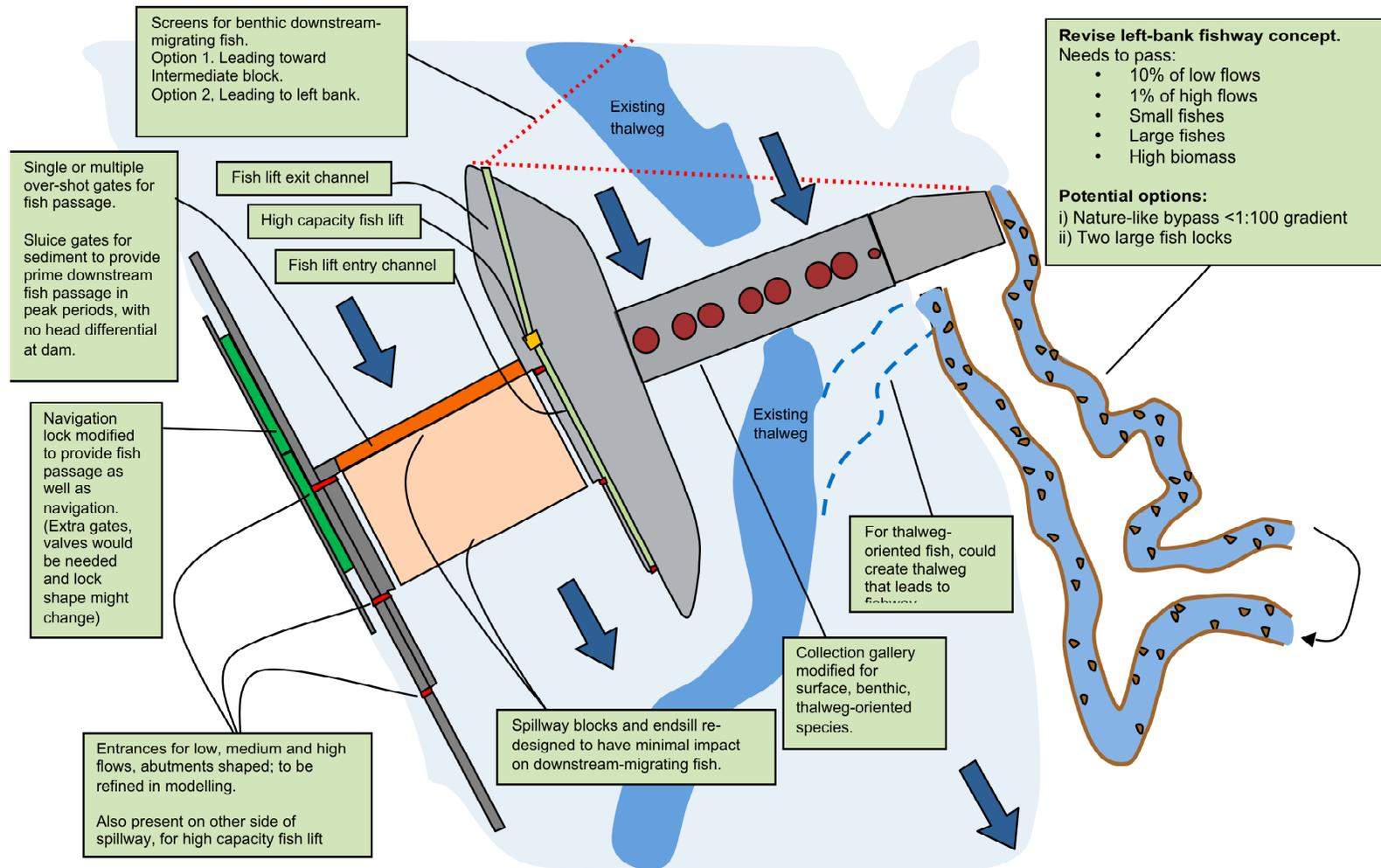
Figure 8: Fisheries Expert Group recommendations for adapting the fish bypass design at Xayaburi dam.
