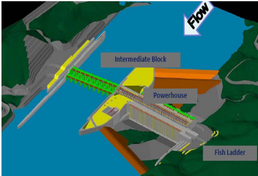
**Figure 6: Second phase of construction proposed in the design documents**
