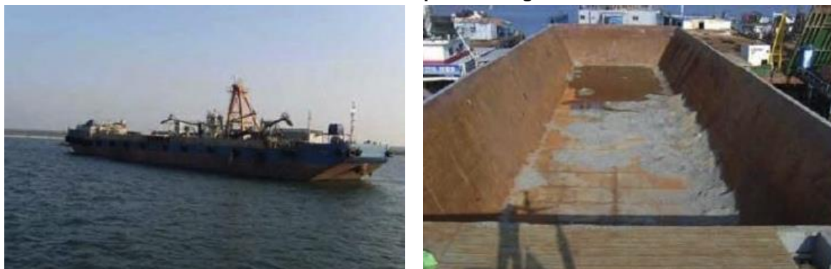
A. Examples of typical coastal aggregate barges with a single open hold. Photos: TOTAL
