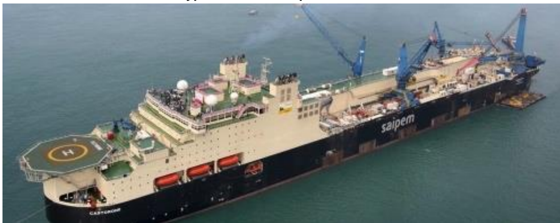
Plate 4.9 – Typical Offshore Pipeline Installation Vessel
