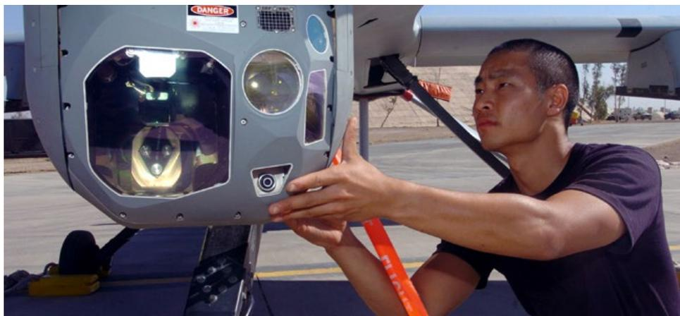
The sensor pod on a Predator drone contains sophisticated cameras, radar, and electronic tracking equipment. Credit Cohen Young, US Air Force
