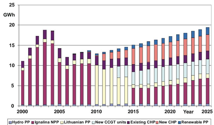
Fig. 14.4. Forecast of electricity generation (new nuclear power plant is commissioned in 2015)
