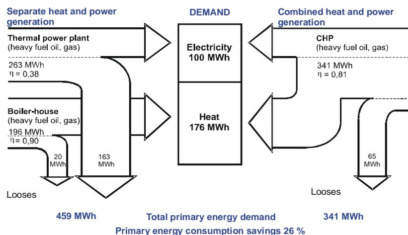
Fig. 8.1. Energy flows for combined and separate heat and power generation
