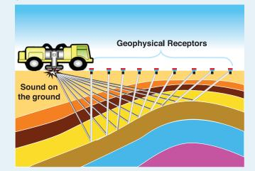
The receptors record the signals that are used to produce detailed images of the earth.
