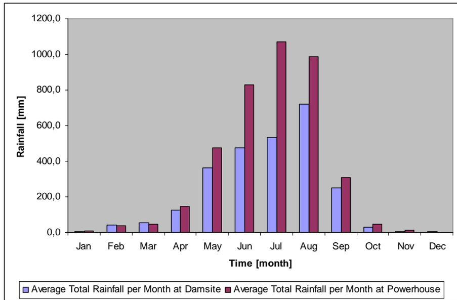
Figure 4-4. Average monthly rainfall measured at Theun-Hinboun damsite and powerhouse from 1999 to 2006 (THPC-EMD)
