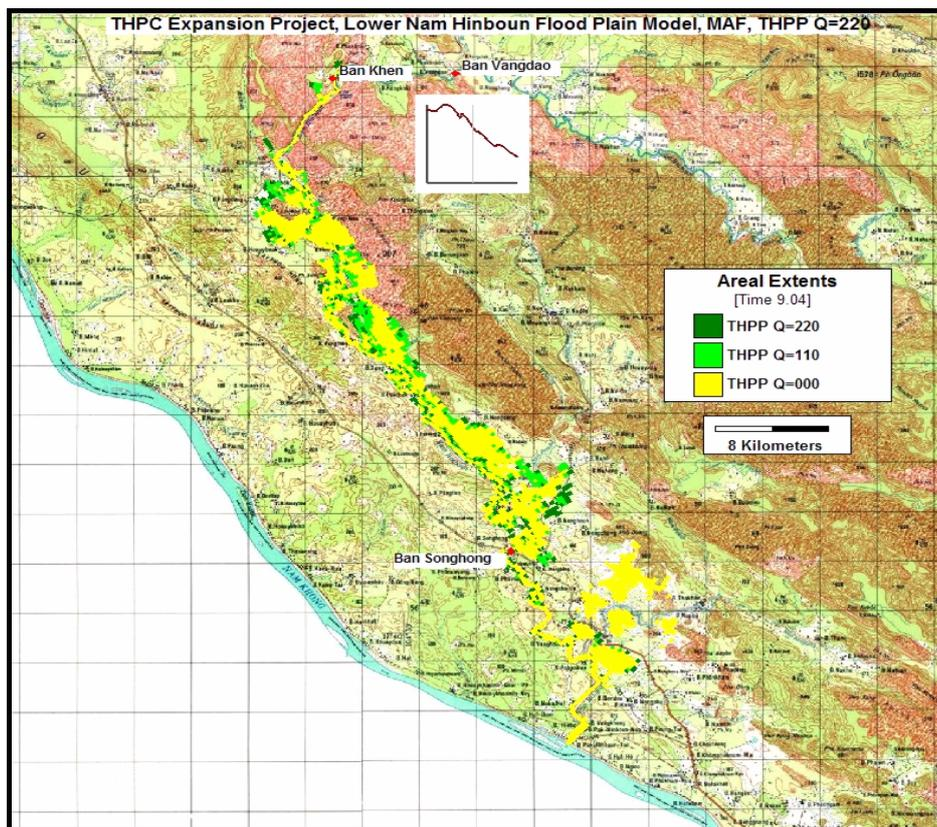
Figure 6-3 Mean Annual Flood in Lower Nam Hinboun for different THPP water releases
