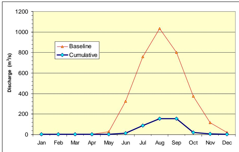
Figure 8-2. Impact on flow in Nam Kading just downstream the Theun-Hinboun weir.
