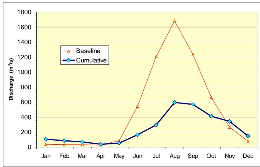
Figure 8-4. Impact on flow in Nam Kading downstream NT1 Dam.
