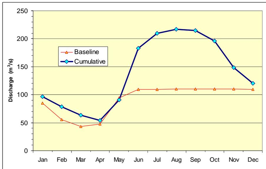
Figure 8-3: Cumulative impact on discharge through Theun-Hinboun Power Station.
