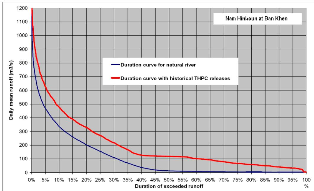
Figure 4-14. Flow duration curve of Nam Hinboun at Ban Khen with and without the THCP operation (SWECO 2007)
