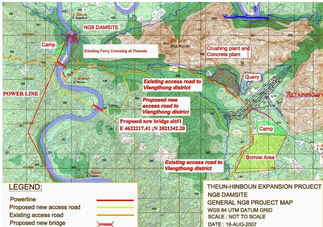
Figure 3-4. Auxiliary and Ancillary Project Features in the dam site zone. Quarries, spoil tips, retaining dyke, etc.
