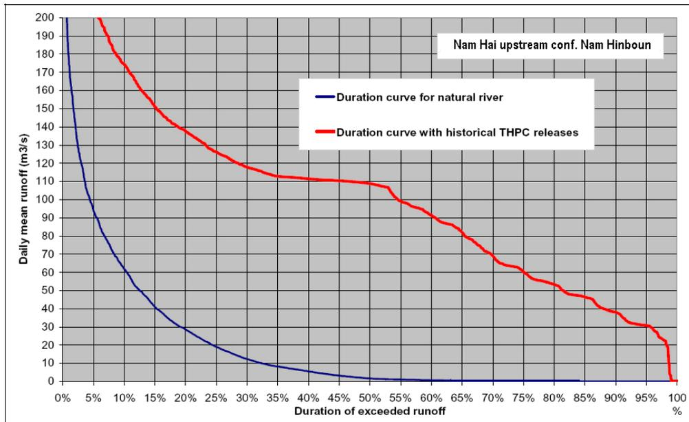
Figure 4-13. Flow duration curve at Nam Hai before its confluence with Nam Hinboun with and without the THPP operation (SWECO 2007)
