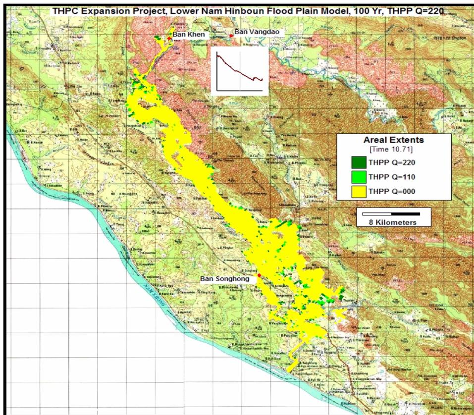
Figure 6-4 100 Year Flood in Lower Nam Hinboun for differnt THPP water releases.
