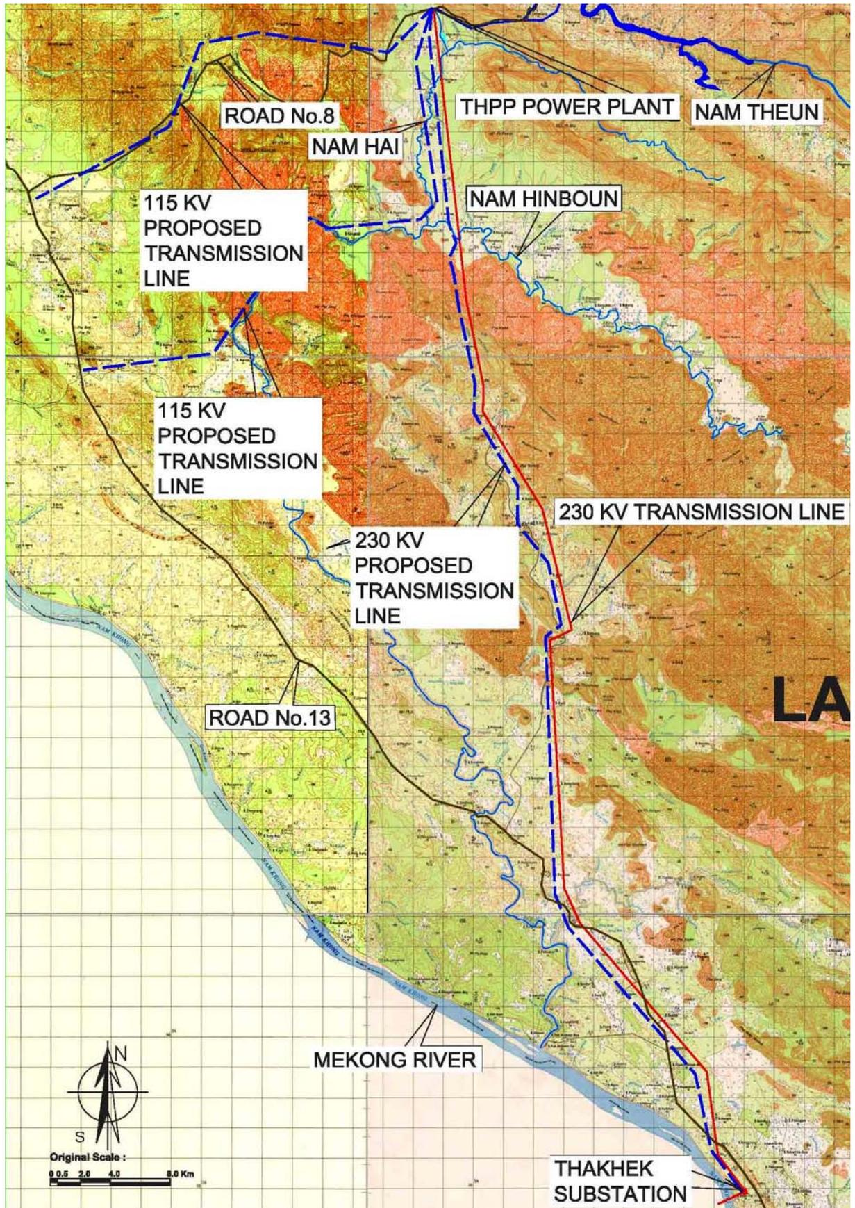
Figure 3-6. High voltage transmission line corridor
