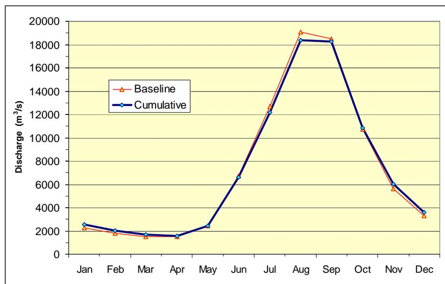
Figure 8-5. NT2, THXP and NT1 impact on Mekong discharges at Savannakhet, downstream the Xe Bangfai confluence.
