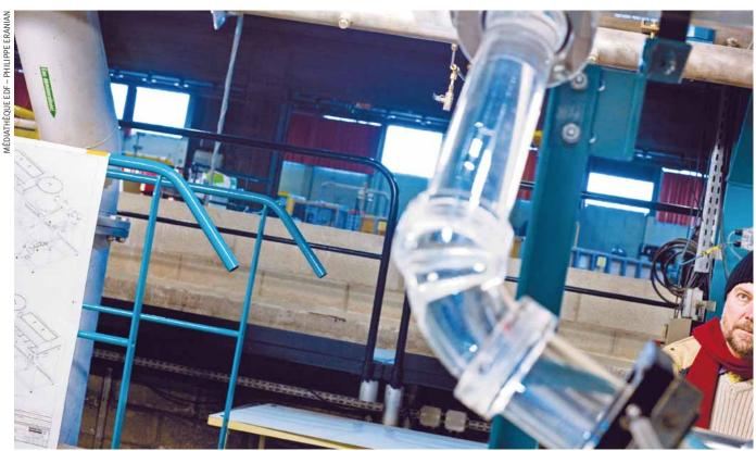
EDF R&D is improving the performance and safety of the Group's facilities. Here, work being done on the boucle CARERRA to optimize the reactor cooling system during shutdown.
