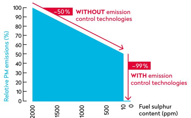
Emission control technologies become fully effective only at 10–15 ppm or less. This is why it is impossible to clean the air without first removing sulphur from fuels. | SOURCE: UNEP and ICCT
