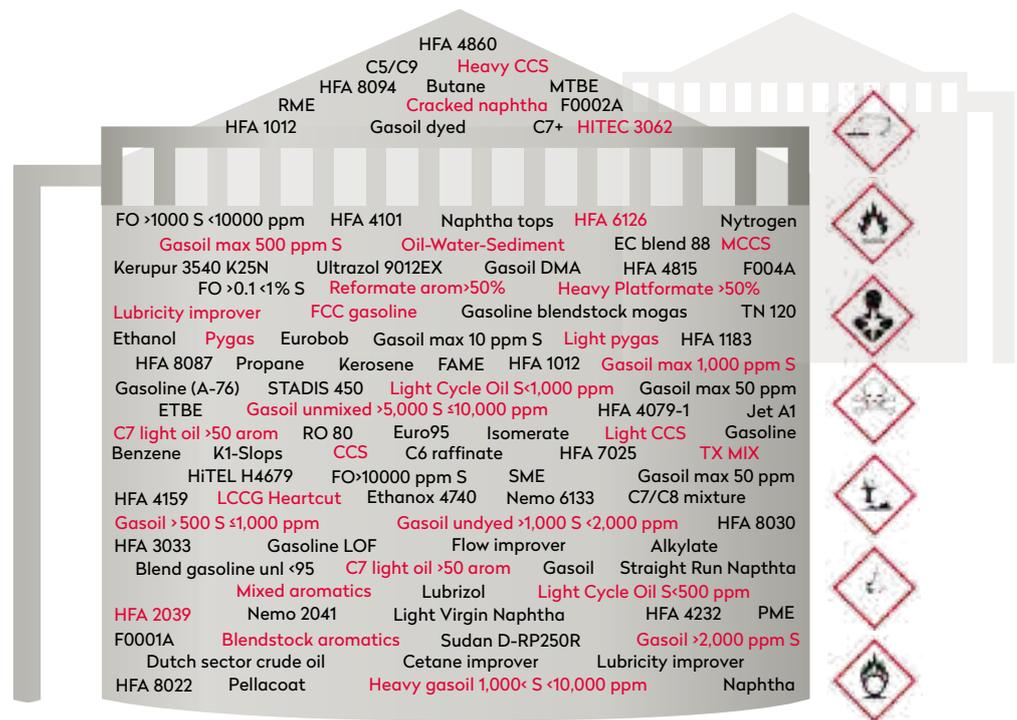
This figure provides a summary of different products, blendstocks and additives. Tricky (potentially unhealthy) blendstocks or additives that might be used for blending into African Quality fuels, are marked in red.
