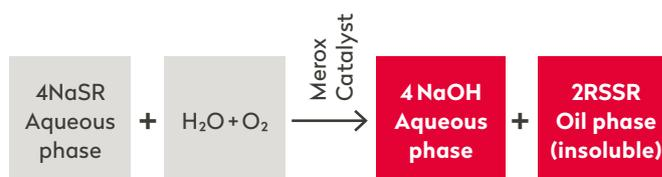
MEROX treatments and caustic soda washing are not only used by refineries. Others also perform these processes, for example, at tank terminals or aboard tankers at sea. Sometimes these others intentionally perform only the first step so that the process is then a caustic wash. As we saw in chapter 2 in which we de-
