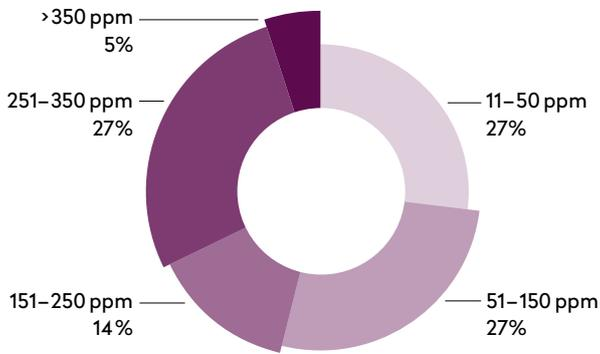
Figure 6.8 –Aromatics concentration ranges of the gasoline samples
