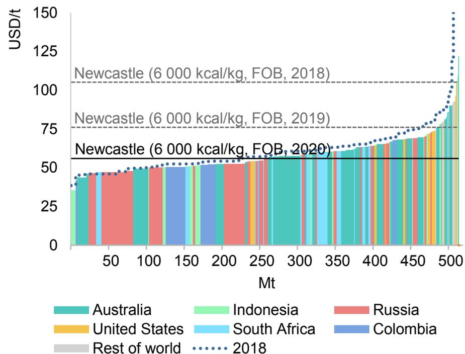
Indicative low calorific (< 4 500 kcal/kg) thermal coal FOB supply curve 2019 and average FOB marker prices
