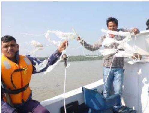
Due to a lack of “Oil Snare” sorbent dragging line, as usually used, a prototype has to be built (see above photos). It consists of a 20m long rope (diam. 0.5 cm), weighted with 2 weights (<1 kg) – one at the extremity and 7 metres before- and equipped with some stripes of oleophilic fabrics (i.e. on which the oil is prone to adhere) - each 50 cm - that were available on the mission boats (PPE, and big bag).
