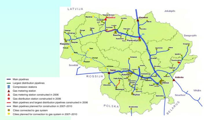
Fig. 16.1. Natural gas transmission network in Lithuania
