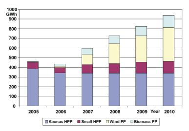
Fig. 14.1. Electricity production from renewable energy sources
