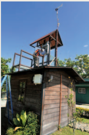
PT Freeport Indonesia installed a state-of-the-science continuous air monitoring system to detect the possible presence of mercury sometimes associated with artisanal mining activities.
