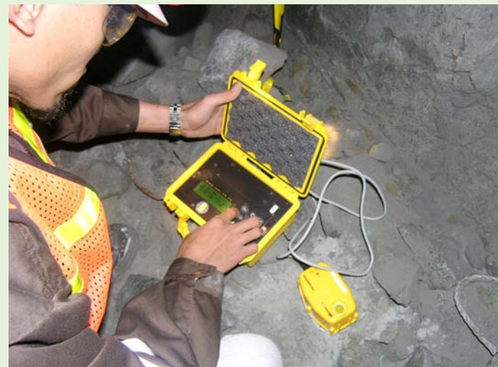
A machine measures blast vibration in the underground mine.
