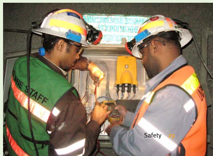
A machine measures blast vibration in the underground mine.
