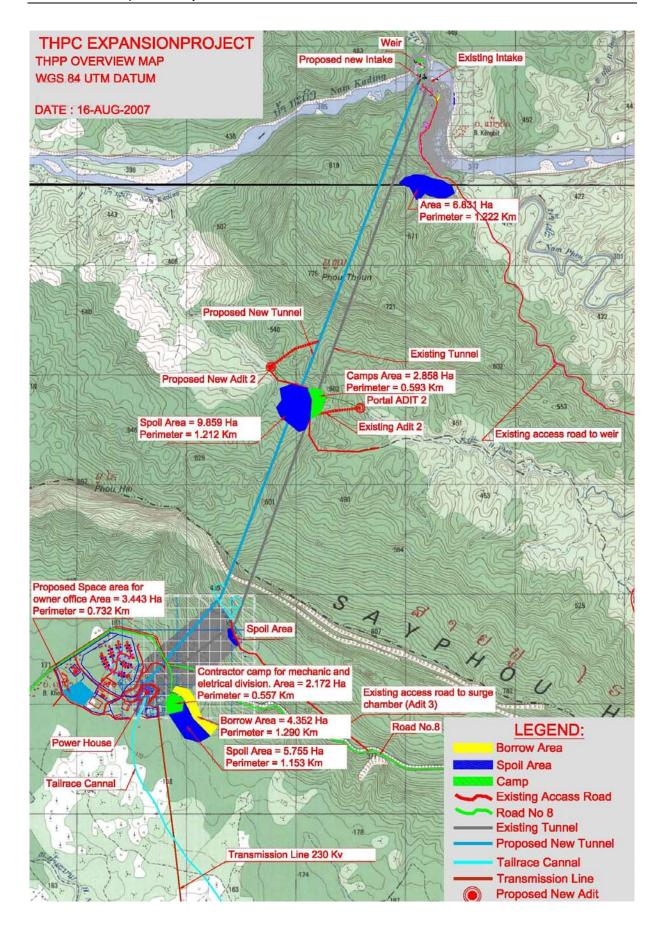
Figure 3-5: Location of Intake, Diversion Tunnel, Adits, Roads and Spoils for THXP.
