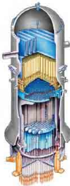
Figure 5.2-3. Schematic of the reactor core of the ABWR ( www.gepower.com/prod_serv/products/nuclear_energy/en/new_reactors.htm ).
