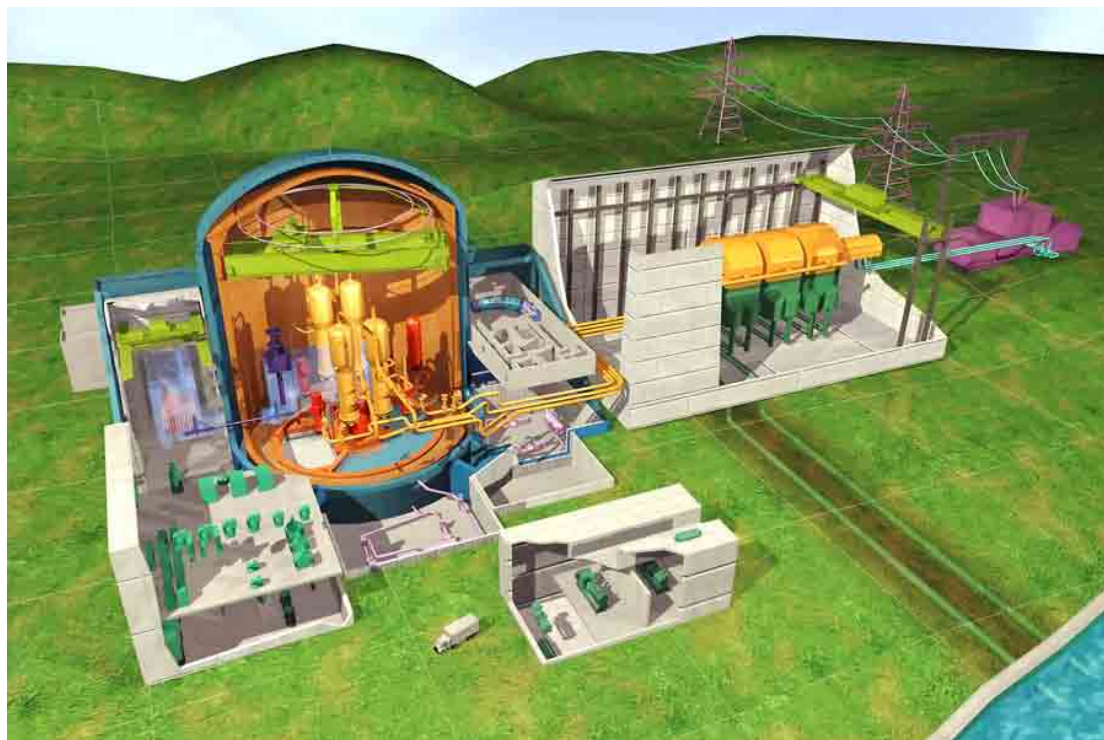
Figure 5.2-1. Schematic of the principal buildings of an EPR ( www.areva-np.com ).
