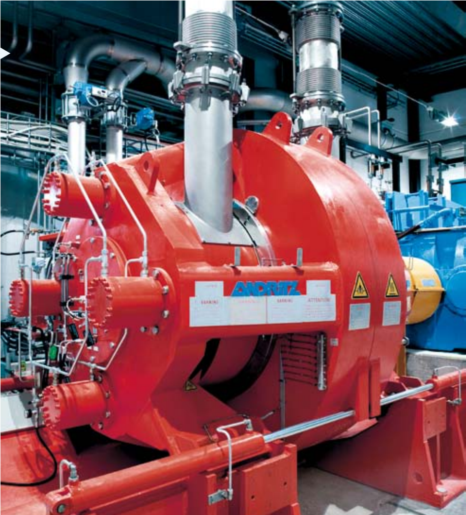
The world's largest LC Refiner was successfully commissioned in the Braviken pulp mill, Sweden. This refiner significantly reduces energy consumption.
