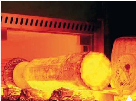
Car bottom annealing furnaces are used for heat treatment in forging mills, foundries, heat treatment-only plants in the steel industry, as well as in the non-ferrous metal industry.
