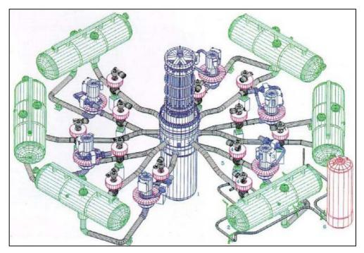
Figure 10 - Primary circuit representation with the six coolant loops
