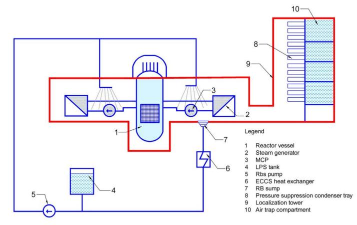
Figure 12 - Schematic diagram of VVER-440/213 containment system
