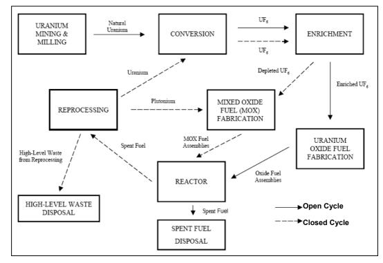
Figure 16 - Open and closed fuel cycle
