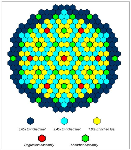
Figure 14 - Layout of the first core for MO34
