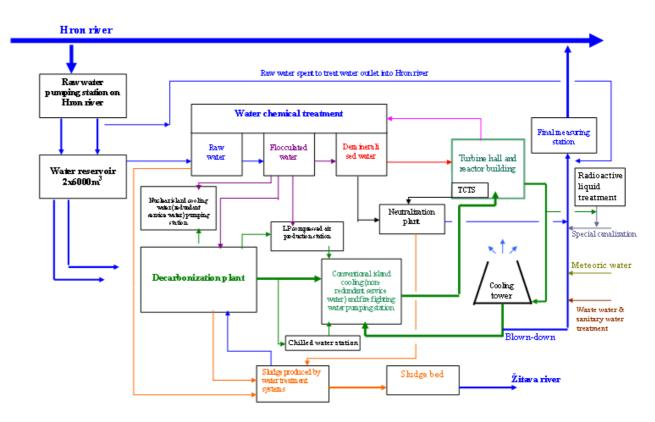
Figure 32 - Water cycle for the Mochovce NPP.
