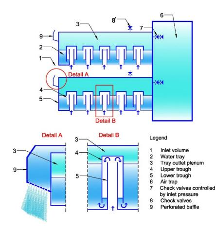
Figure 13 - Details of bubbler condenser's trays and air trap compartment of VVER-440/213 containment system
