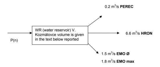
The excessive flow not being used by the NPP, Perec or the small water power station (SWPS) is driven through Veľké Kozmálovce dam to the Hron channel. The SWPS can abstract and let flow only the water that is not used by the NPP. The outflow to Perec is realized through a special object or through the SWPS and other outlets. Water abstraction by the NPP is realized by a special object.
