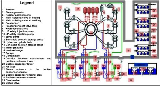
Figure 11 - Safety system scheme
