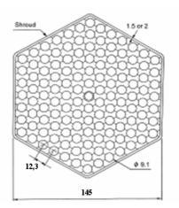
Figure 15 - Fuel assembly cross section
